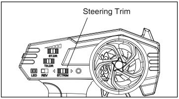
The steering trimmer is used to adjust the central position of servo if the vehicle can't run straightly. Switch left / right to adjust servo central position to left / right.
