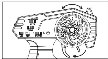
Rotate the steering wheel clockwise / counter-clockwise while pulling the trigger to make a right / left turn.
