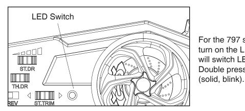
For the 797 series with LED, short press the button to turn on the LED. When the LED is on, each short press will switch LED colors, until it turns off.
