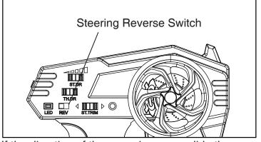
If the direction of the servo is wrong, slide the steering reverse switch to the opporsite direction.
