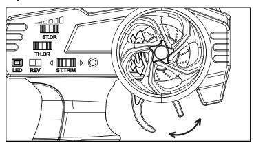
To move forward the boat, pull the throttle trigger as shown. To move backward the boat (if with reverse feature), push the throttle trigger as shown.
