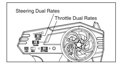
Adjust the steering dual rates to gain the proper steering ratio. Switch left / right to turn by a smaller / larger angle.
